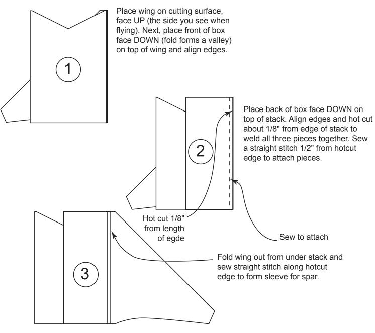
Place second wing on cutting table, face UP. Place box-wing stack from step 3 on top and align wing and box edges. Hotcut together and sew as in steps 2 and 3 to complete kite assembly.
